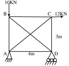
4. Analyse the rigid jointed frame shown in fig. by flexibility method using force transformation approach. Draw BMD and elastic curve. 16marks
