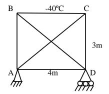
8. Analyse the given beam by force method of analysis, having temperature change in members AB and BC of 15°C. Depth of the beam is 400mm,  $\alpha = 10 \times 10^{-6}$ / ° C, E = 30000 N/mm<sup>2</sup>, I = 50 x  $10^{6}$  mm<sup>4</sup>.
